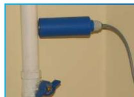
**Magnetic base of ADM sensor** is also used for pipe diagnostics in hard-to-reach places and on the pipes of small diameter.
